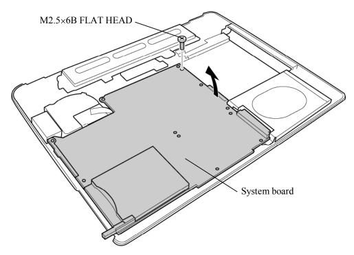
Figure 4-27 Removing the system board (2)
